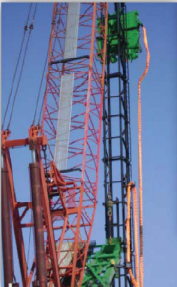
Group and protect hoses on pile driver against stretching and tearing.
