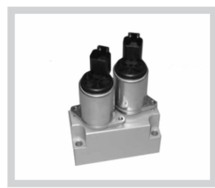
The PVHC is an electrical actuator module for main spool control in PVG 32 and PVG 100. The actuator uses two current controlled proportional pressure-reducing valves. PVHC does not use the known PVE internal closed loop control technology, and does therefore not offer any kind of fault monitoring system, neither active nor passive.
