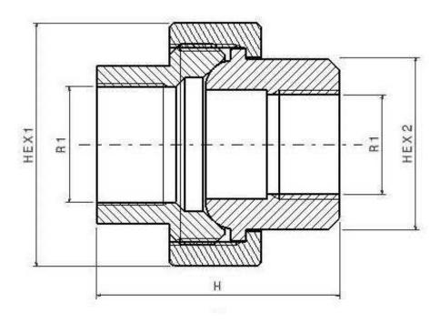
**Norms:** Male thread according to EN10226-1 Female thread according to ISO 228-1
