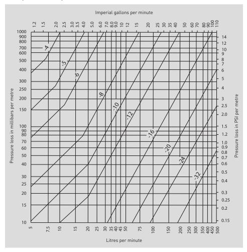
Based on: fluid viscosity 20 cSt specific gravity 0.875
