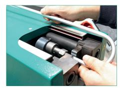
The assembly head differs from the standard model by the holder for the cutting ring assembly socket being moved upwards, shortening the distance from the tube axis in the assembly socket to the upper edge of the machine from the standard 77 mm to 31 mm.
