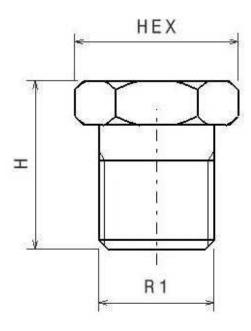
**Norms:** Male thread according to EN10226-1 Female thread according to ISO 228-1
