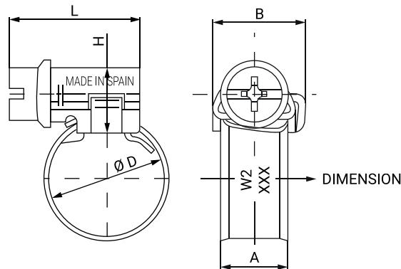
The ASFA L7 is the smallest worm-drive hose clamp in the Mikalor range and, dare we say it, in the world. This clamp has been developed for use in applications where a standard clamp cannot be used due to a shortage of space. It is manufactured using the same technology and production processes as the current 9mm and 12mm ASFA ranges and is subject to the standards and quality controls specified by ISO 9001 and IATF 16949.
