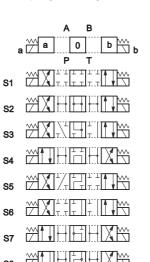
Type **SA\***: 1 solenoid side A 2 positions (central + external) with spring centering
