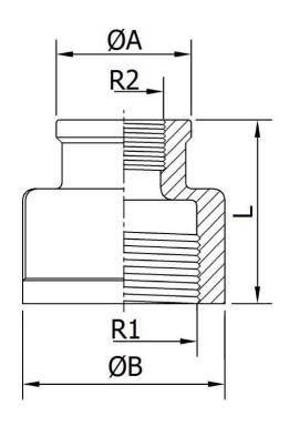
**Norms:** Male thread according to EN10226-1 BSPT Female thread according to ISO 228-1 BSP
