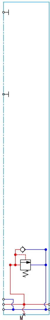
Maximum pressure for P- and T- port
