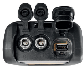
PPC-04-plus with 2 sensor inputs for max. 2 analogue STAUFF Sensors
