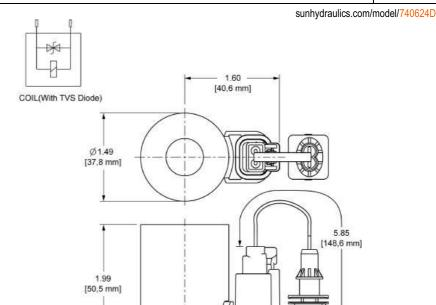
This 740 Series Coil configuration uses a connector adapter kit to provide the required termination.
