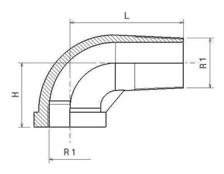
**Norms:** Male thread according to EN10226-1 BSPT Female thread according to ISO 228-1 BSP
