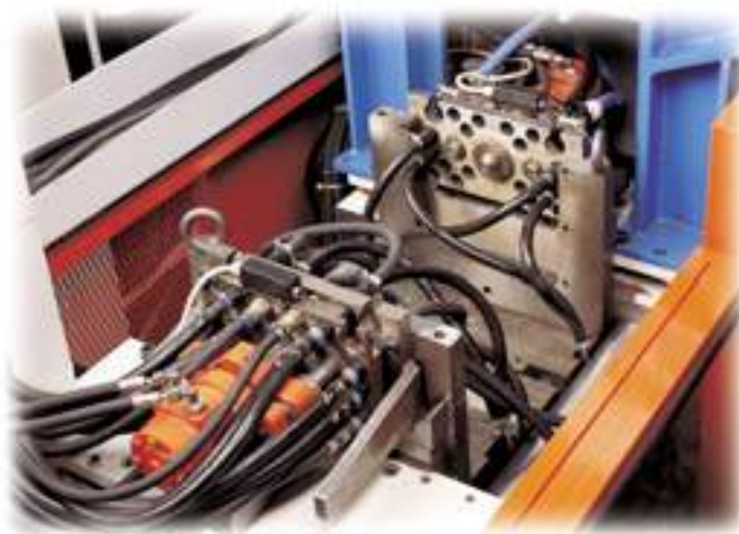
Multiconnection for quick moulds replacement. Moulding machine. Up to 18 hydraulic, electrical and pneumatic lines.
