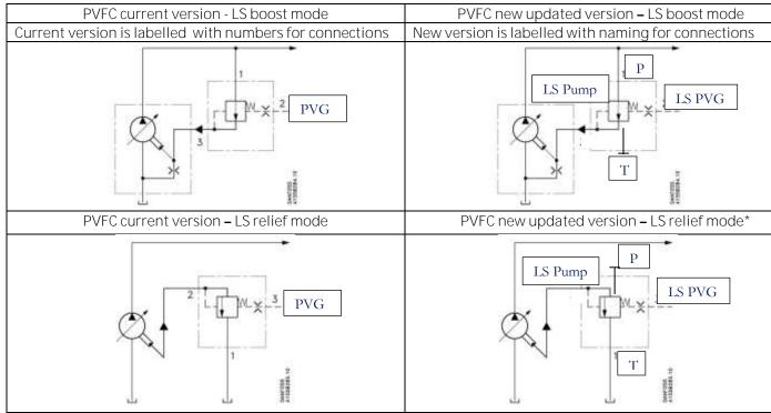
\*Default, the new version will be delivered and set up for LS boost. If LS relief mode is required, the plug in the T-port is moved to the P-port and T-port is connected to Tank
