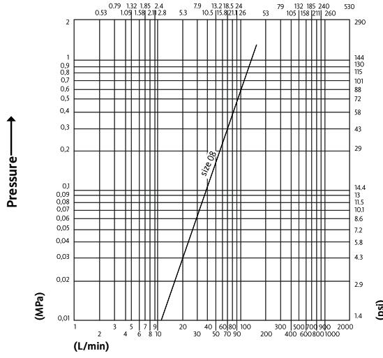
Test performed according to ISO 18869
