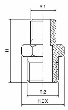
**Norms:** Male thread according to EN10226-1 BSPT Female thread according to ISO 228-1 BSP
