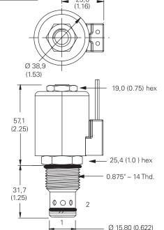
Torque cartridge in aluminum housing 47-54 Nm (35-40 ft lbs) Note: When solenoid valve is ordered as cartridge only, coil nut is included.
