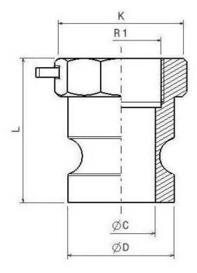
**Norms:** Male thread according to EN10226-1 Female thread according to ISO 228-1
