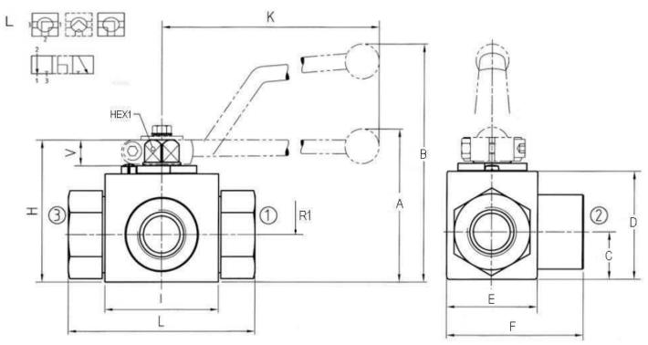
Lever: Zn Tmin/Tmax: -20°C/+100°C Standard o-ring: NBR Ball seat: POM
