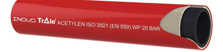
**Application:** A flexible hose for the transport of acetylene. For welding and cutting, for arc welding using shielding gas and related processes. Also suitable for H, CO2, AR, & N. (Not suitable for LPG, MPS and CNG).
