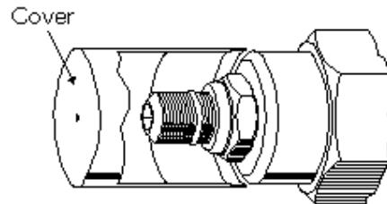
Sun's tamper resistant cover is a zinc plated steel cover which press-fits onto the L Control cartridge shoulder. Valves may be ordered in this configuration from Sun by specifying a C control in the model number. The pressure setting must be specified at the time of the order and the setting will be stamped on the cartridge hex. Sun kits for replacement parts or field conversion are available.
