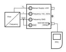
The measured data are transferred to the Hydraulic Testers directly with the normal CAN or analogue Connection Cables.
