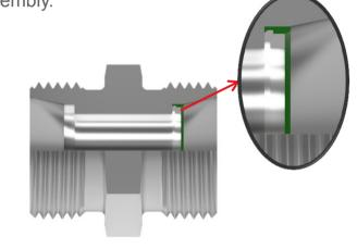
Place the FSSR ring onto the cylindrical end of tube. Tighten the nut by hand and further with a suitable spanner for appr. 120  $^{\circ}$  / 2 Flats. A significant increase of force shows the end of assembly.
